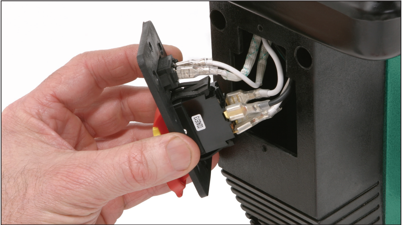
Figure 32. G9969 Switch Wiring.
